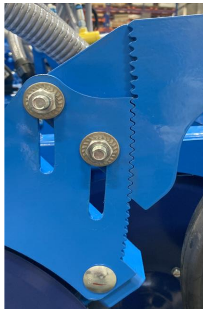
Depth of sowing coulters by 4 cm
