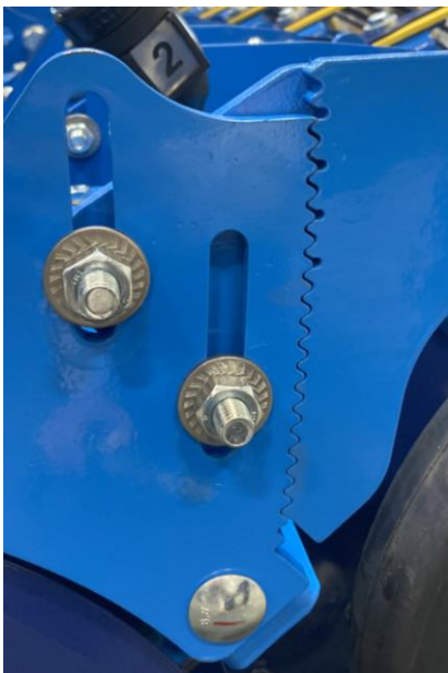
Depth of sowing coulters by 1 cm.
