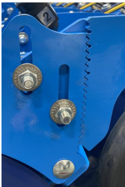
Depth of sowing coulters by 1 cm.
