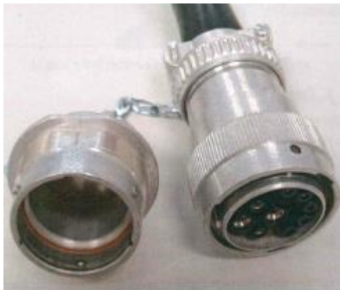
Picture. 4 - Connection socket on the tractor
