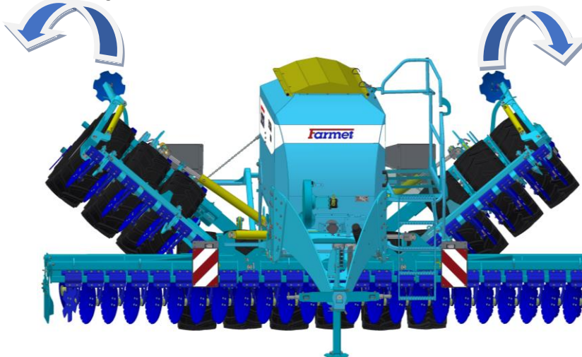
Picture 25 - Unfolding the machine
