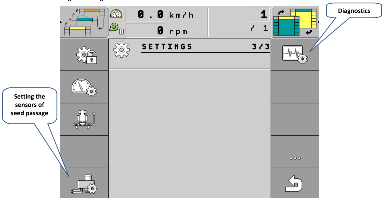
Picture 22 – Setting the sowing sensors
