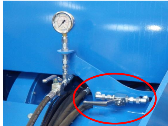
Picture 31- Ball valve, front section, position ON
