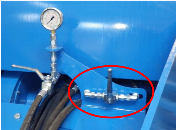
Picture 30 - Ball valve, front section, position OFF
