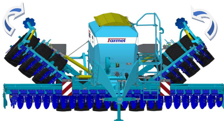
Picture 28 – Folding the machine
