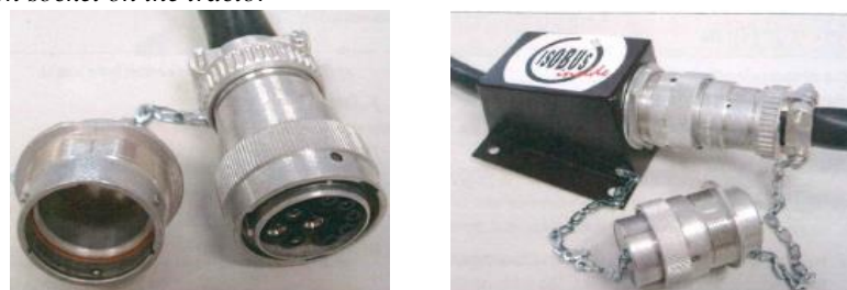
Fig. 7 - Connection socket on the tractor
