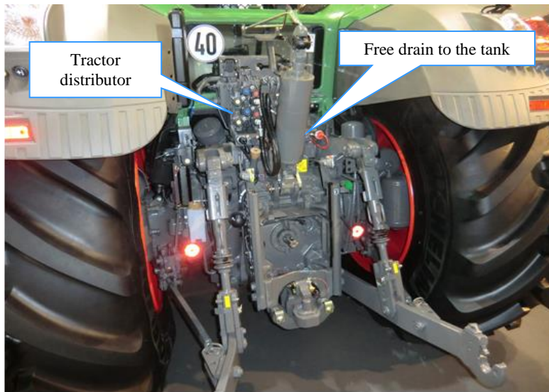
Fig. 9 – Position of quick couplings in the tractor
