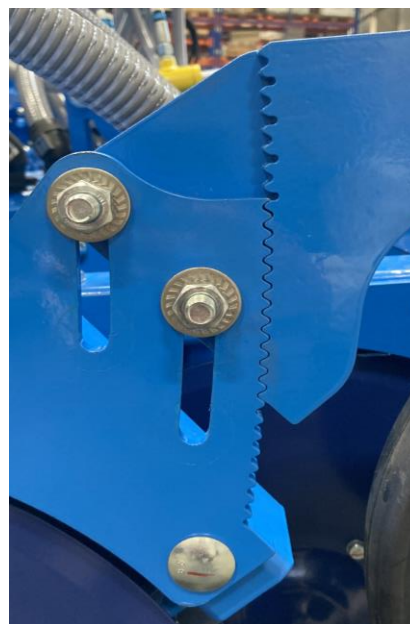
Depth of sowing coulter by 4 cm
