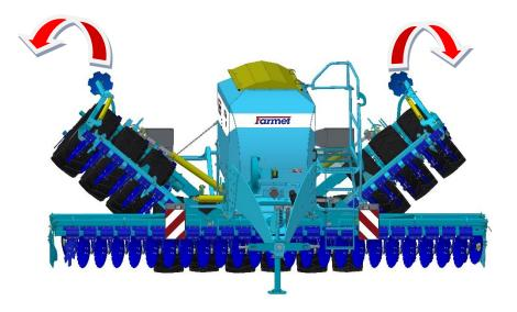
5. When the machine is completely unfolded and the circuit has been pressurized, confirm the task of unfolding (C). The machine is now completely unfolded and the sowing application can be activated.
