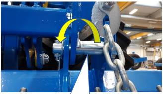
Remove the spacer sleeve, transfer the seeding units using the screw, place the spacing sleeve on the other side of the brace
