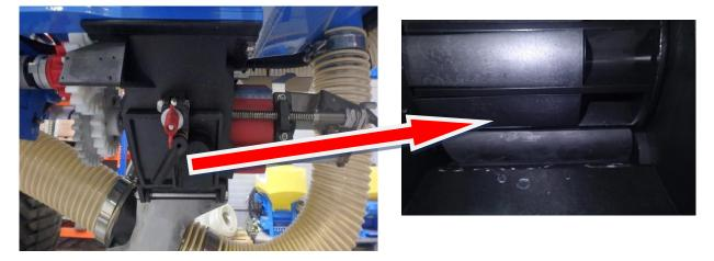
For fine seeds, set the setting roller to position  $\mathbf{0}$  – the container must be cleaned and closed beforehand and the seeding mechanism must be empty. Place the closing valve on the body of the feeder into the cut on the hexagon shaft. This way the roller of the feeder can move only within the range from 0 to 25 mm.
