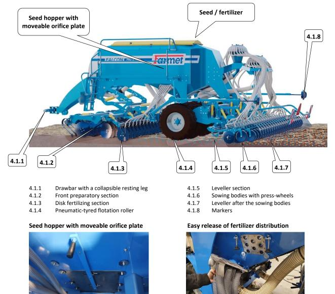
Picture 3.1 – Working parts of the machine **FALCON PRO**
