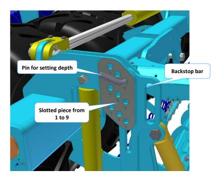
Picture 57 - Openings in the slotted piece
