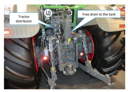
Picture. 6 – Position of quick couplings in the tractor
