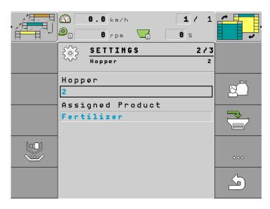
2. Write down the weight that you poured into the hopper (use the rotary knob on the side of the terminal).
