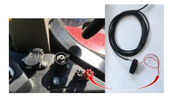
Picture. 4 - Connection socket on the tractor
