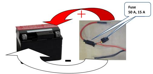
ATTENTION! Check correct polarity of the cable!
