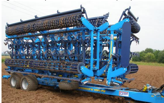
Fig.9 – Auxiliary wheels are in the transport position
