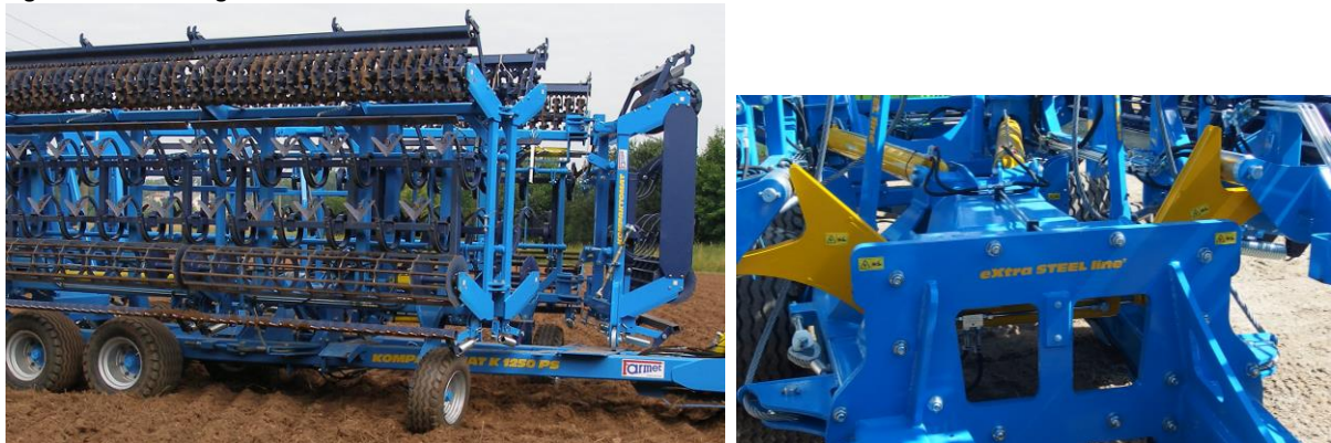
Fig.16 – The working section has reached the catches located on the chassis
