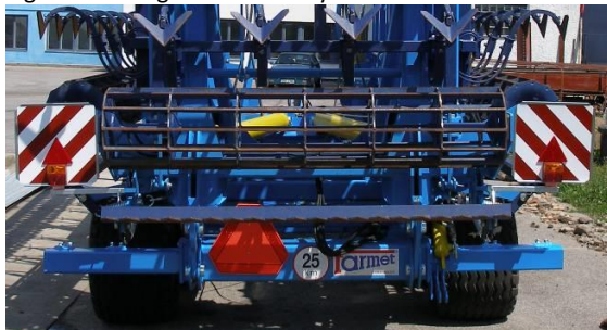
Fig.18 – Placing the rear safety shields
