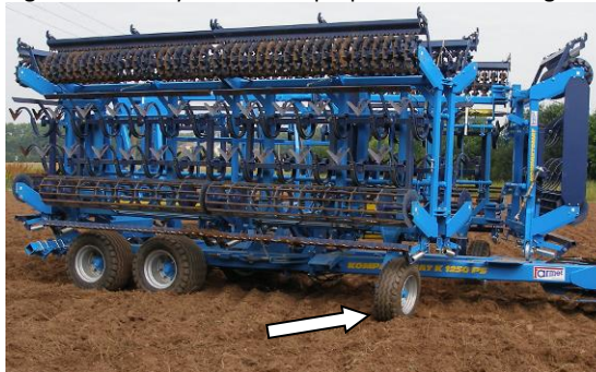
Fig.10 – Auxiliary wheels are prepared for unfolding
