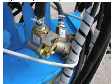
Fig.27 – Quick coupler for brakes
