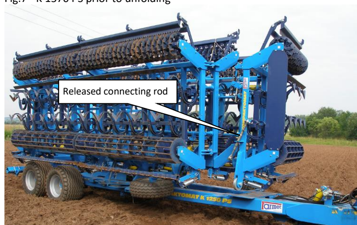
Fig.7 - K 1570 PS prior to unfolding
