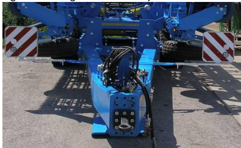
Fig.17 – Placing the front safety shields
