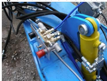
Fig.26 – Hand brake valve control
