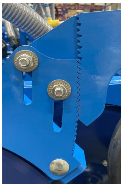
Depth of sowing coulter by 4 cm
