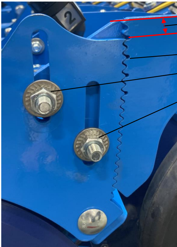
Depth of sowing coulter by 1 cm.
