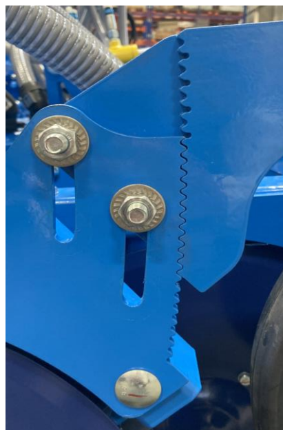
Depth of sowing coulter by 4 cm
