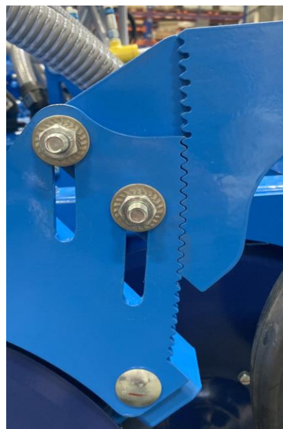
Depth of sowing coulter by 4 cm
