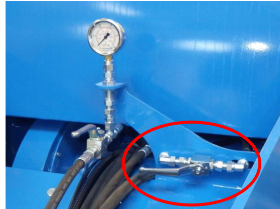
Picture 31- Ball valve, front section, position ON
