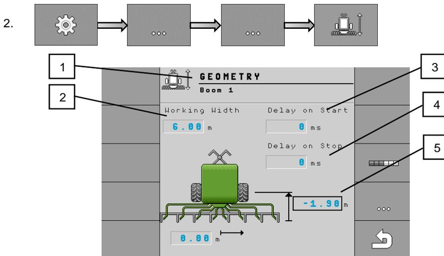
**Note on the point 5:** If the section is behind the axle axis, the value must always be negative (sowing section), if the section is in front of the axle, the value must be positive (fertilization section).
