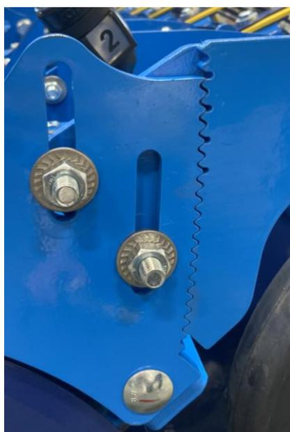
Depth of sowing coulter by 4 cm
