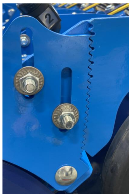
Depth of sowing coulters by 1 cm.
