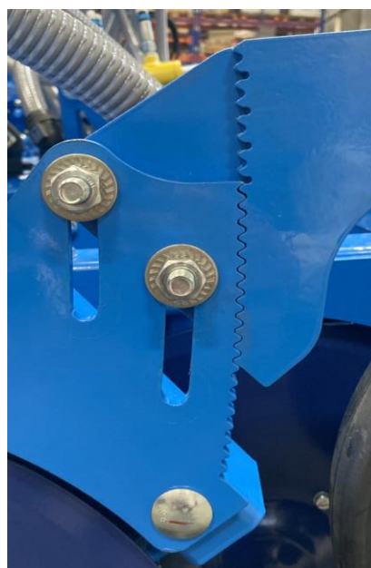
Depth of sowing coulters by 4 cm
