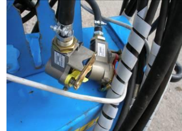
Fig.27 – Quick coupler for brakes
