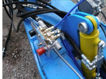
Fig.26 – Hand brake valve control
