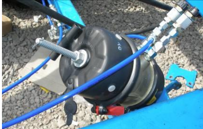
Fig.25 – Spring brake piston rod for hand brake
