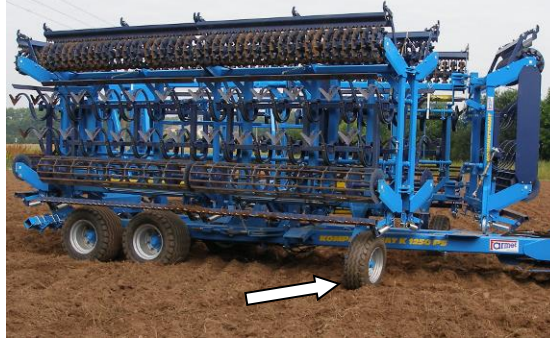
Fig.10 – Auxiliary wheels are prepared for unfolding
