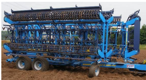
Fig. 30 – Transport position for ploughshare section replacement
