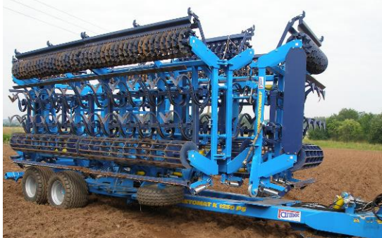
Fig.9 – Auxiliary wheels are in the transport position
