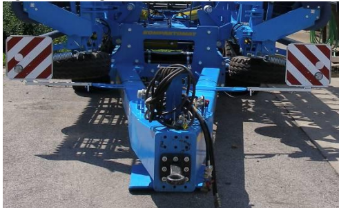
Fig.17 – Placing the front safety shields
