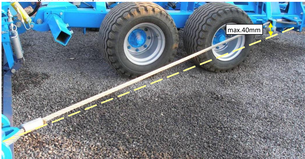
Fig.24 – Pre-stressing of the tractive rope
