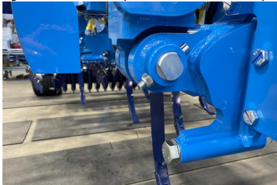
Fig. 7 – Bottom end stops that maintain machine plane
