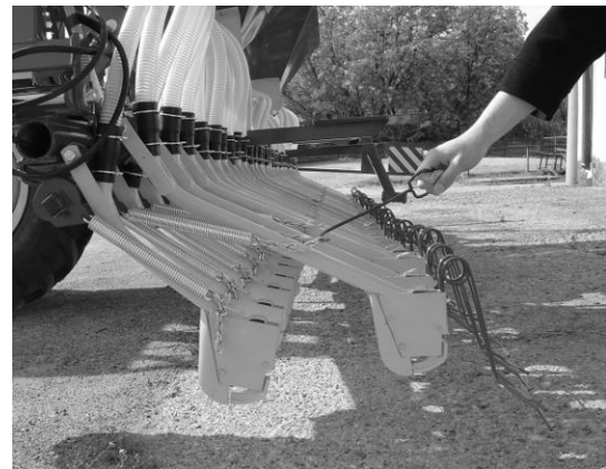
Pic.4 individual change of pressure onto the seeding section
