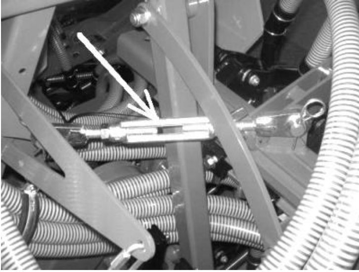
Pic. 12a Locking of folding parts in transport position
