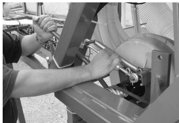
Pic.22 loading of the V- belts, MB
