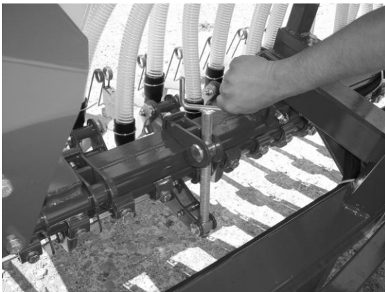
Pic.3 central adjustment of pressure onto the seeding sections
