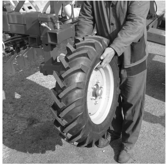
4. Lock the right wheel off, draw it, and turn it per 90°, put into opening and block it.
