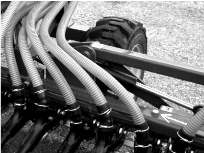
Pic. 12b Locking of folding parts in working position
