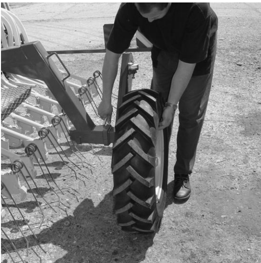
5. Lock the left wheel with head race off, draw it, and adjust the wheel on side of drawbar.
