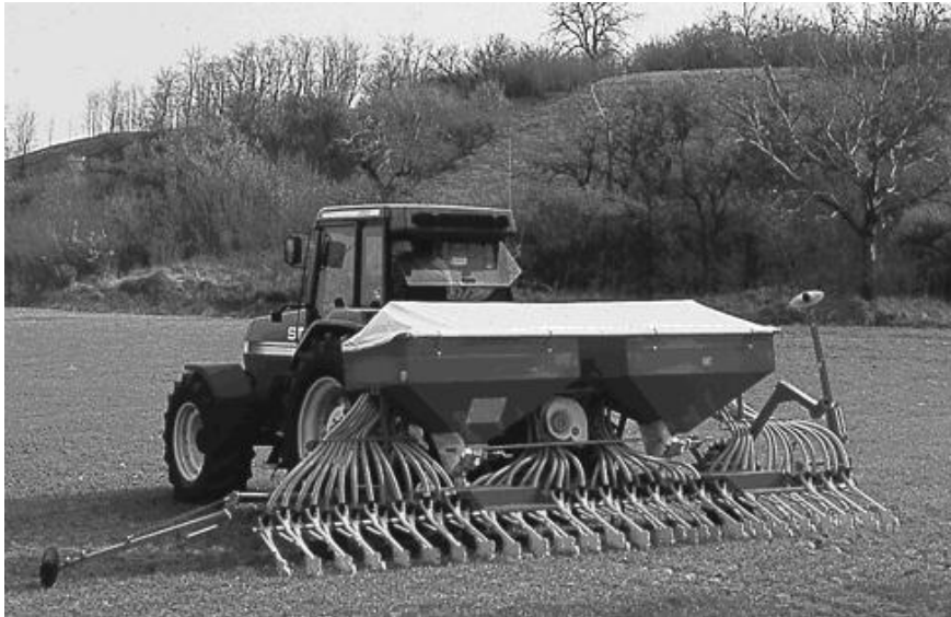
Pic.13 The seed drill MD with working width 6 m
