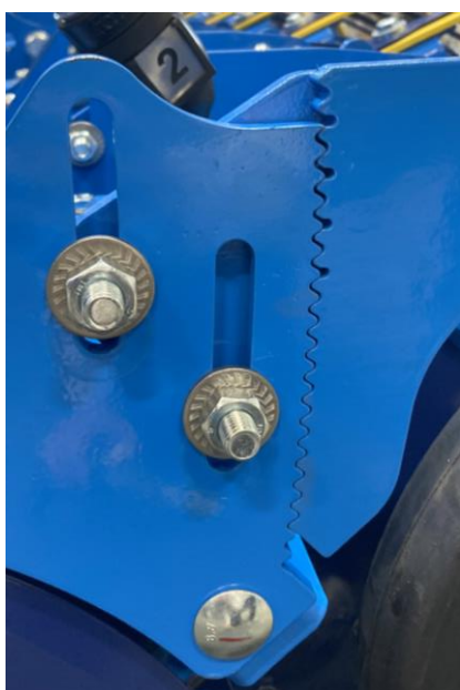
Depth of sowing coulters by 1 cm.
